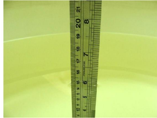
Fig 7.2 Photo of Liquid Height for Body SAR
