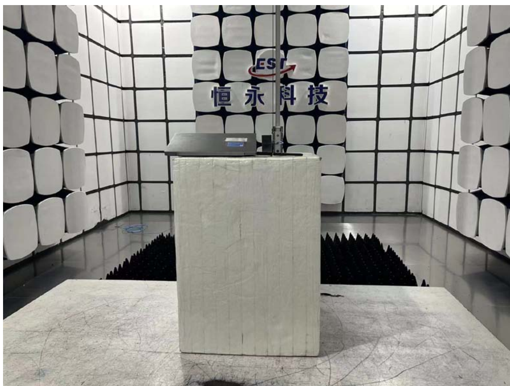
Radiated emission test: Above 1GHz
