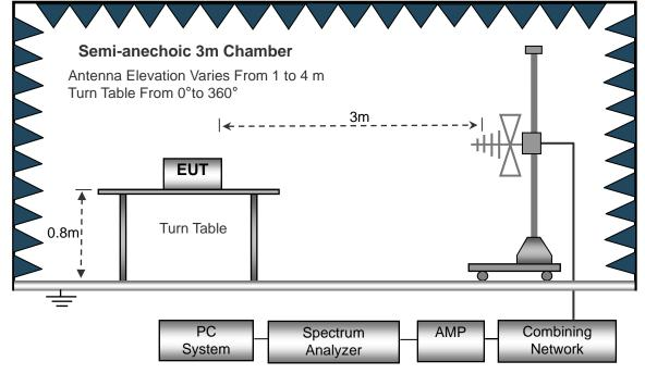
(C) Radiated Emission Test-Up Frequency Above 1GHz
