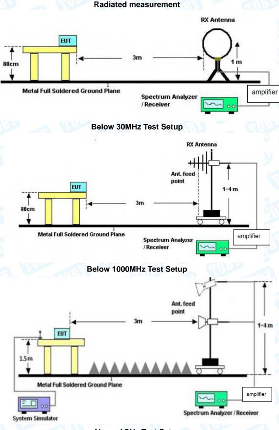
Above 1GHz Test Setup
