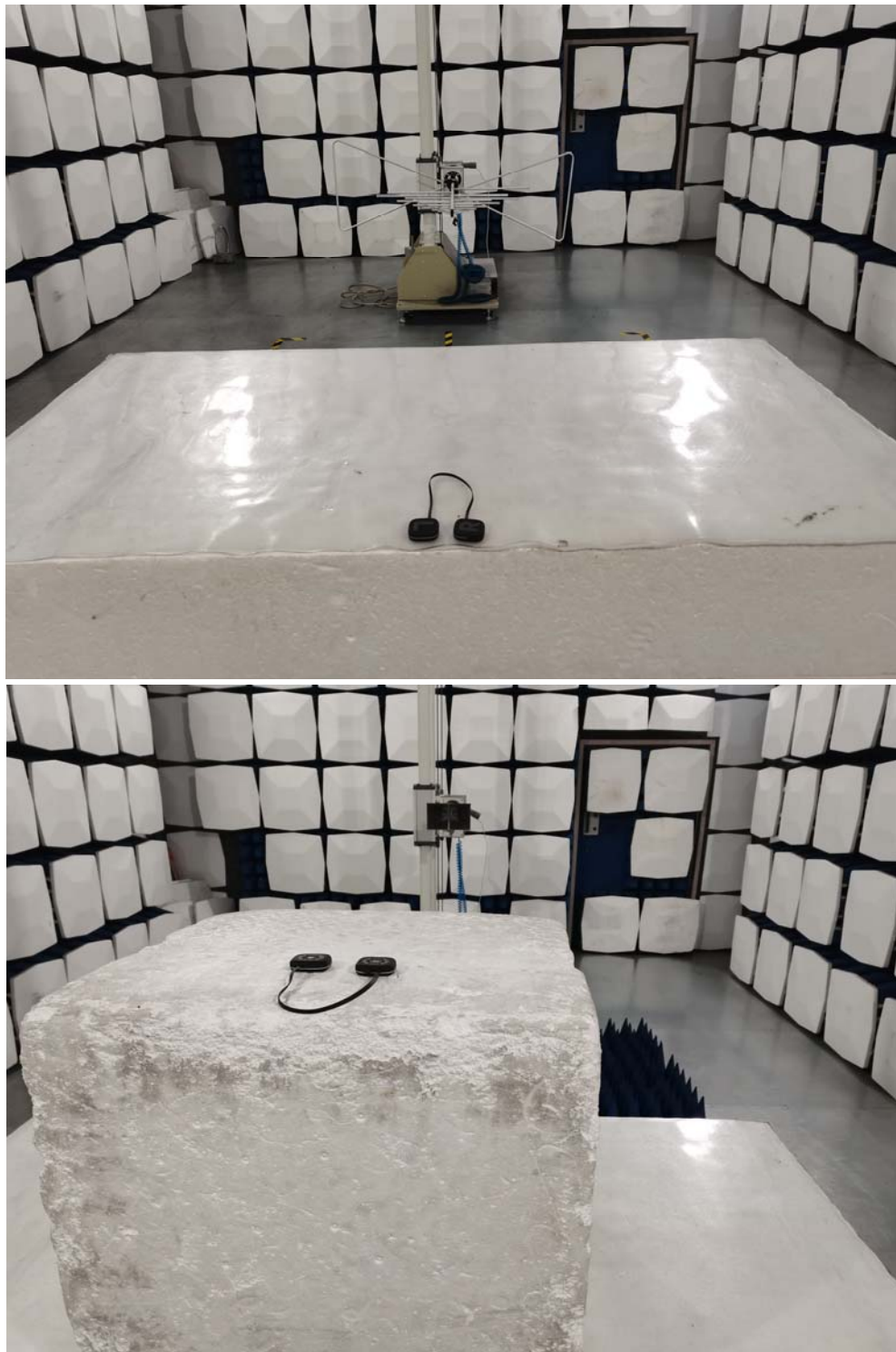
Radiated emission test view
