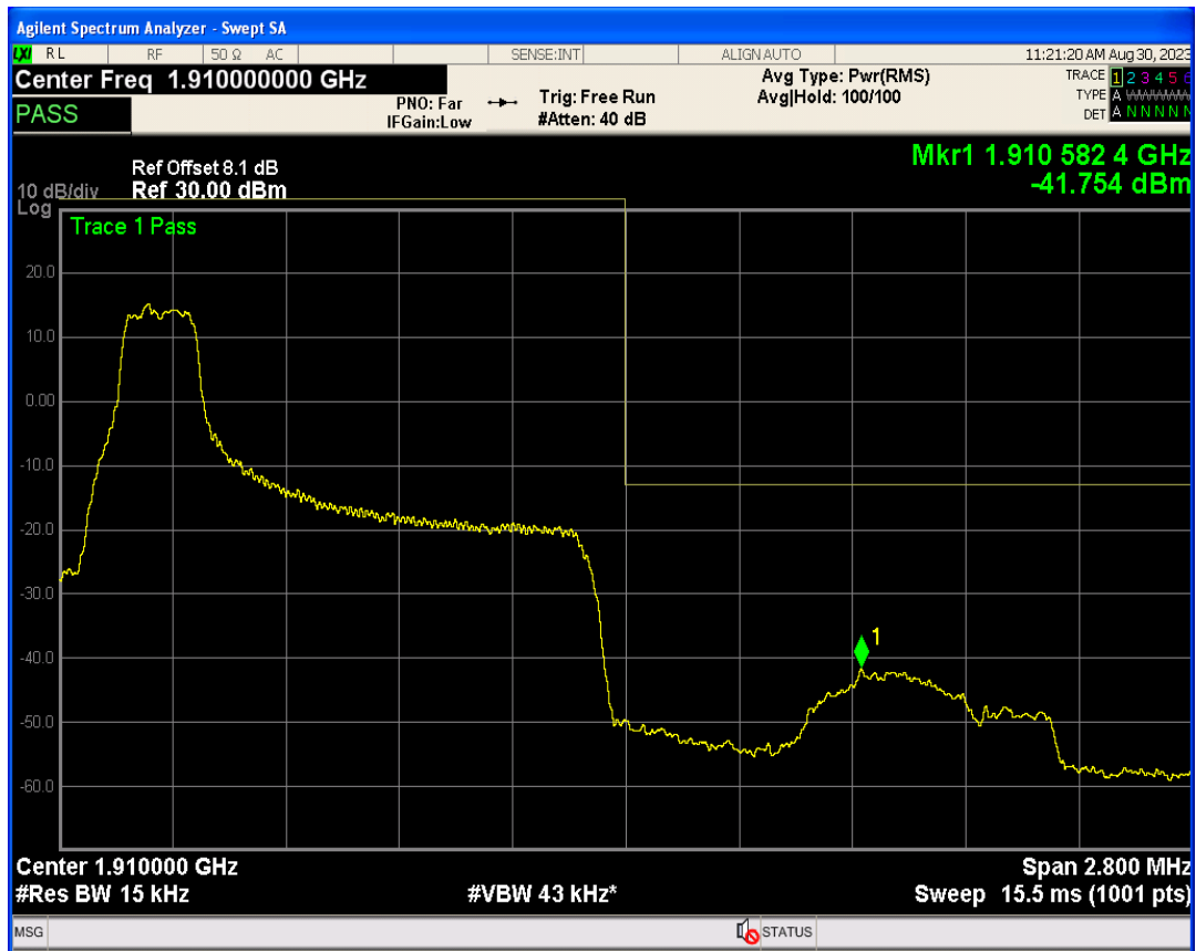
Band2 QPSK BW=1.4MHz Channel=19193 RB Size=1 Position=#Max
