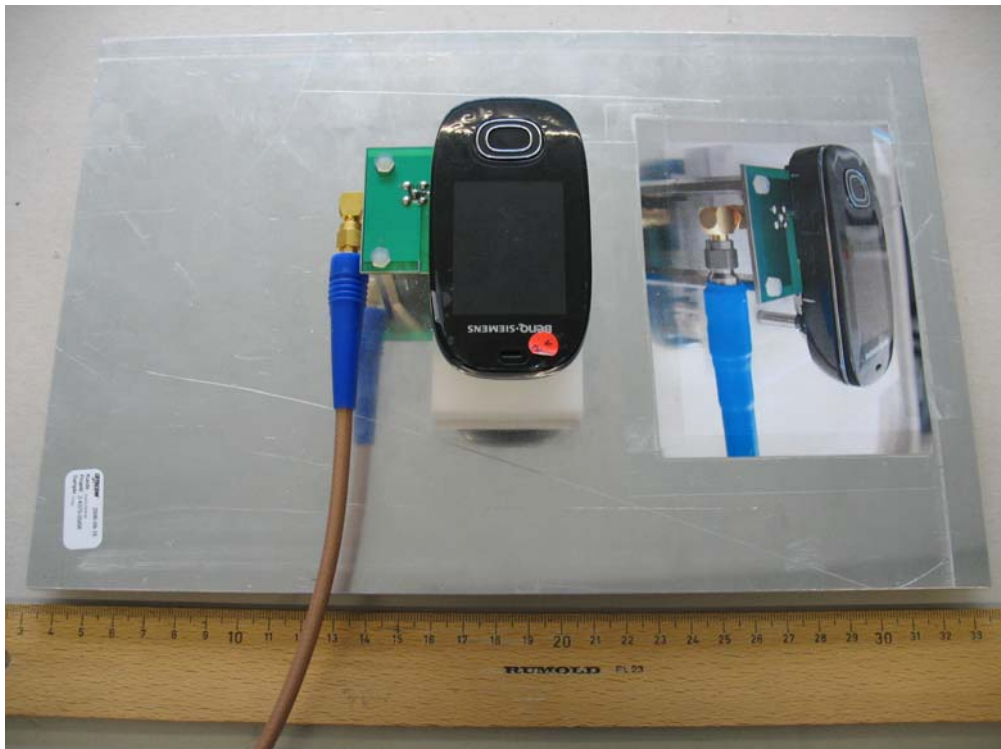
Photo 4: Measurement of Bluetooth conducted
