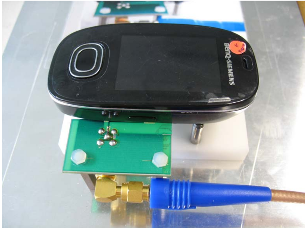
Photo 5: Measurement of Bluetooth conducted
