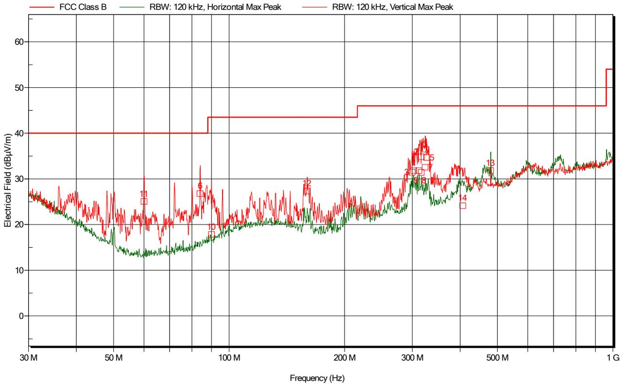
Figure 5.3.7.1: Electric field emissions Plot, 30MHz to 1GHz, 2480MHz Operation
