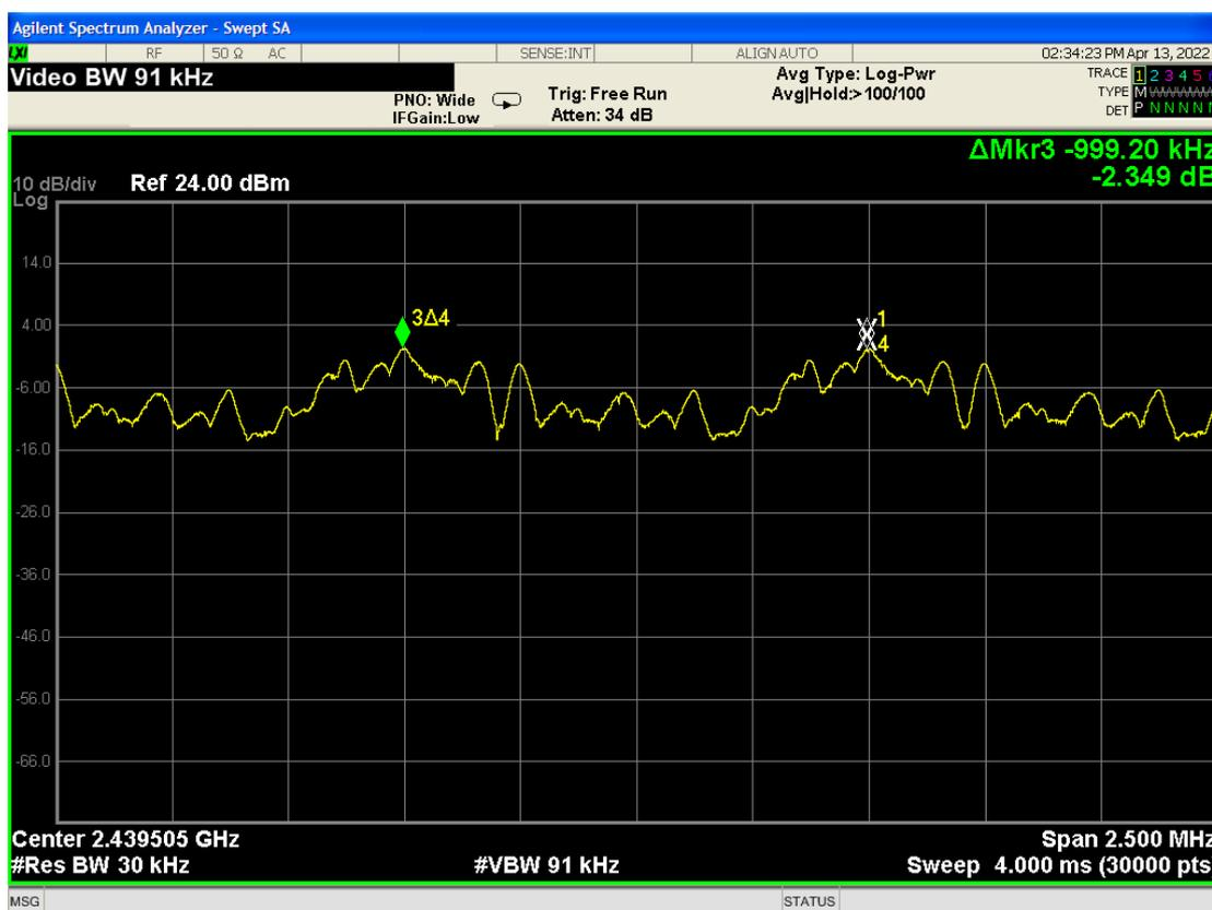
Figure 8.2.7.1: Carrier frequency separation
