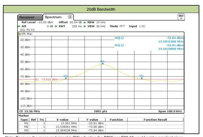
Note: Because the measured signal is CW adjusting the RBW per C63.10 would not be practical since measured bandwidth will always follow the RBW and the result will be approximately twice the RBW.
