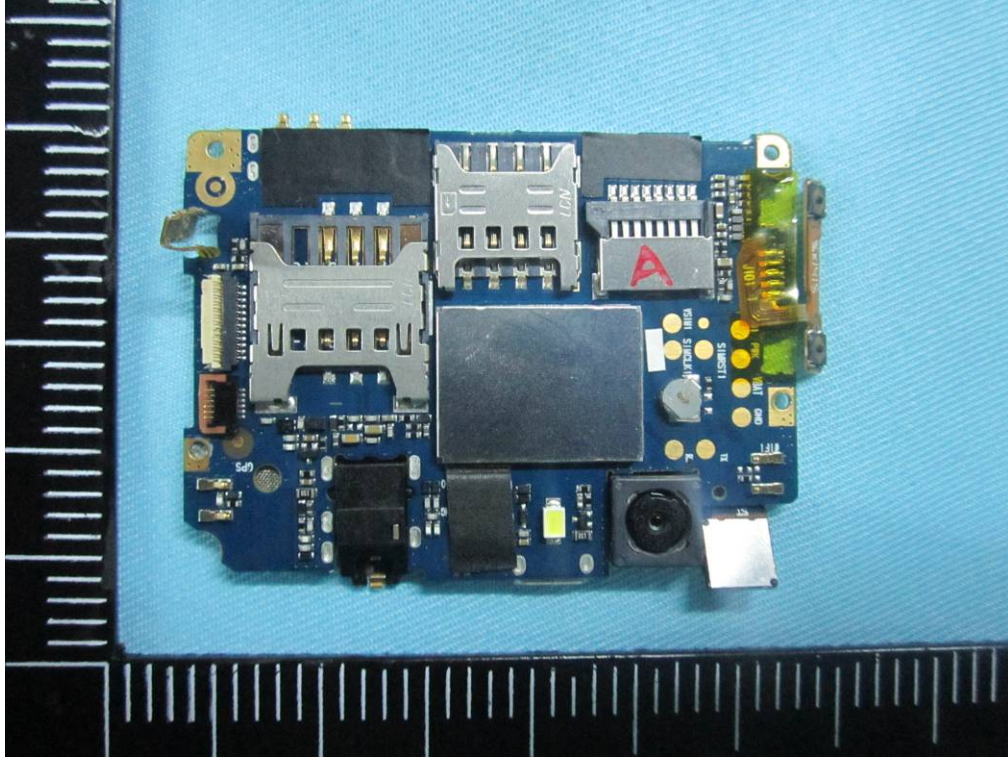
Mainborad With Shielding - Rear View
