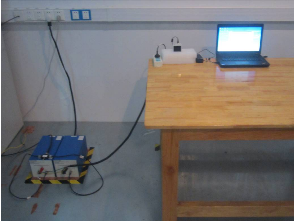
Conducted Emissions Test Setup Front View
