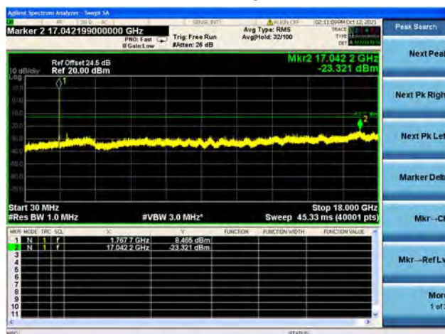
Band66 / 20MHz / High CH / 16QAM
