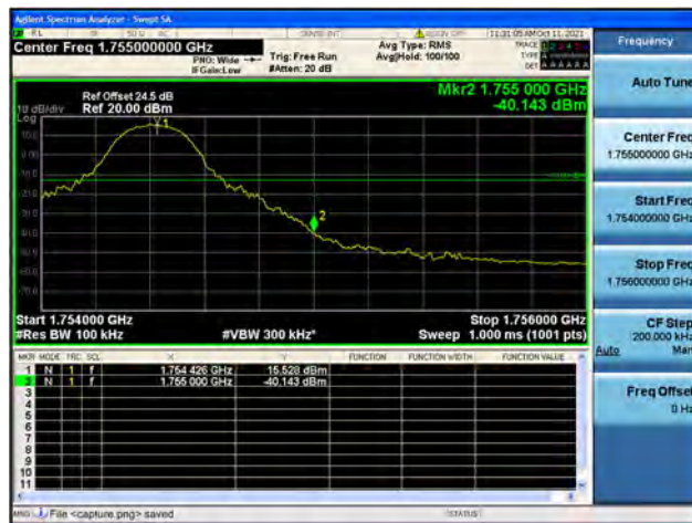
Band4 / 10MHz / High CH / QPSK / 1 RB
