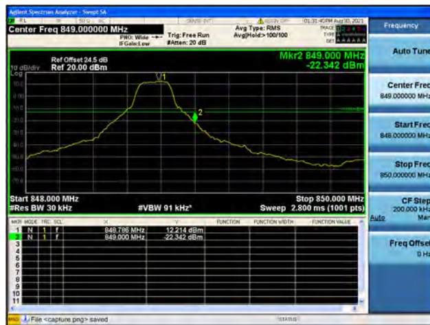
Band5 / 3MHz / High CH / QPSK / 1 RB
