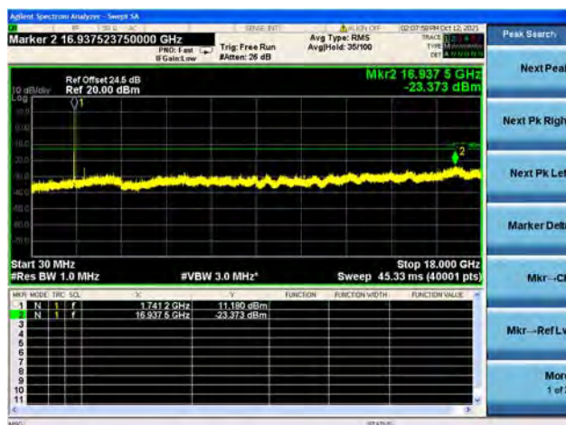
Band66 / 15MHz / Mid CH / 16QAM
