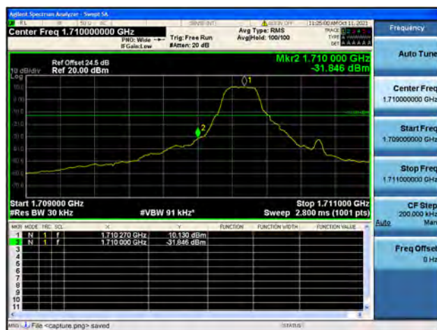
Band4 / 1.4MHz / High CH / QPSK / 1 RB
