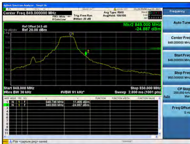
Band5 / 1.4MHz / High CH / QPSK / 1 RB
