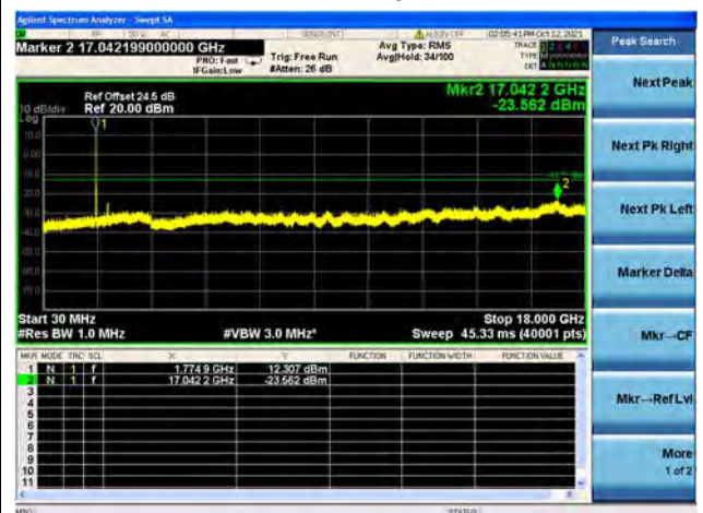
Band66 / 10MHz / High CH / 64QAM
