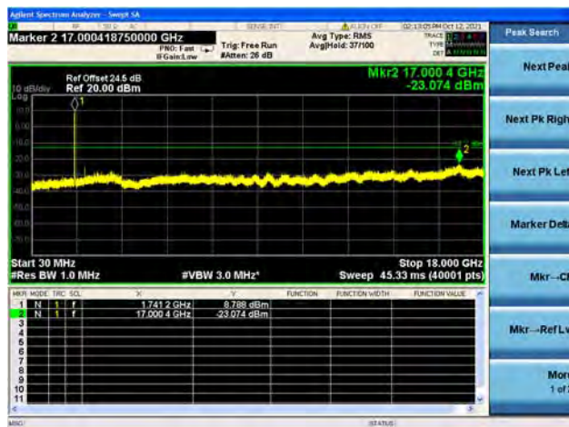
Band66 / 20MHz / High CH / 16QAM
