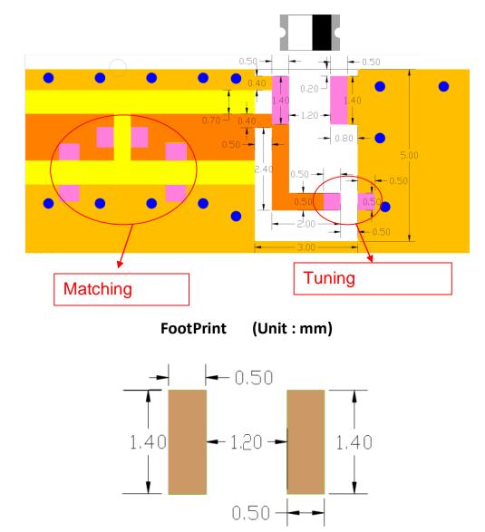
• 2<sup>nd</sup> Layout Dimensions in Clearance area(Size=8.0\*2.5mm)
