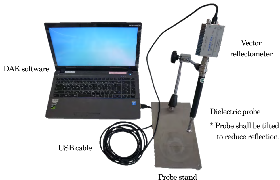
(a) Dielectric Parameter Measurement System
