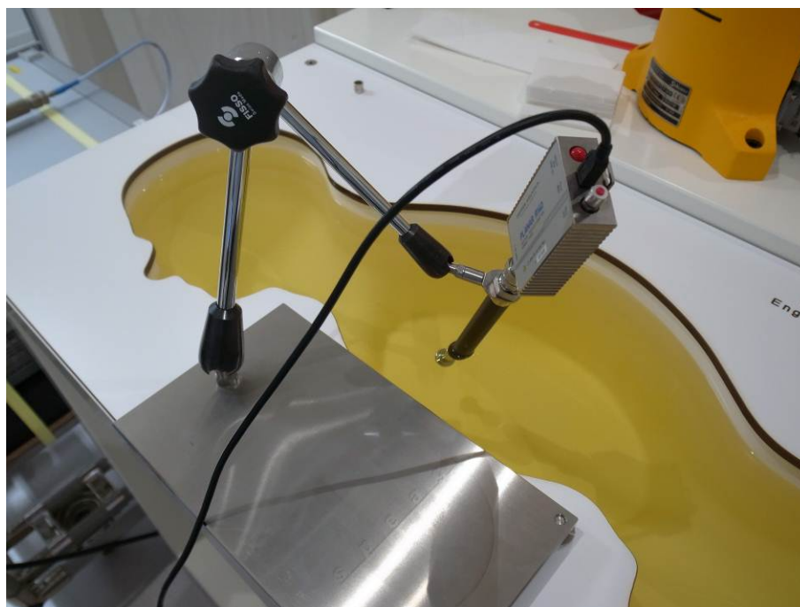
(b) Example Photo: Dielectric Parameter Measurement
