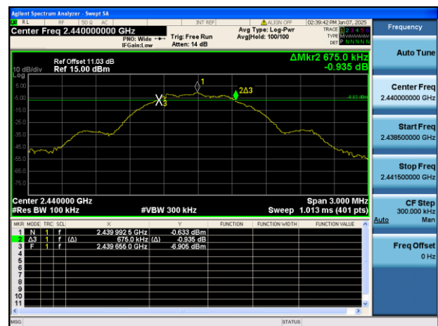
GFSK (BLE 1Mbps) MIDDLE CHANNEL
