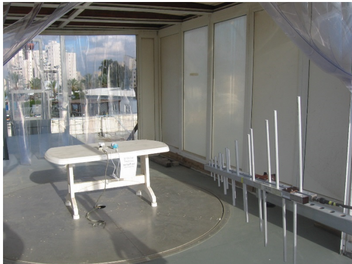
Radiated Emission Test 200-400 MHz
