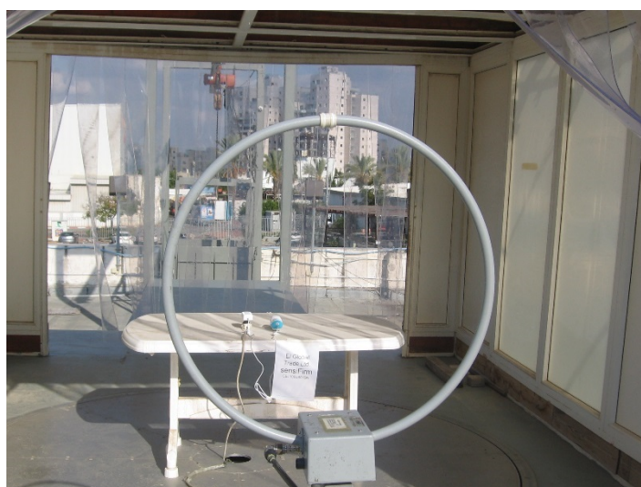
Radiated Emission Test 0.009-30 MHz
