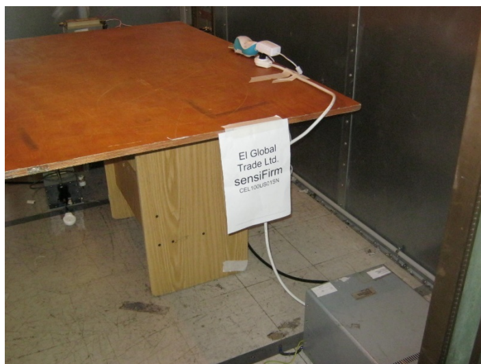
Conducted Emission From AC Mains Test
