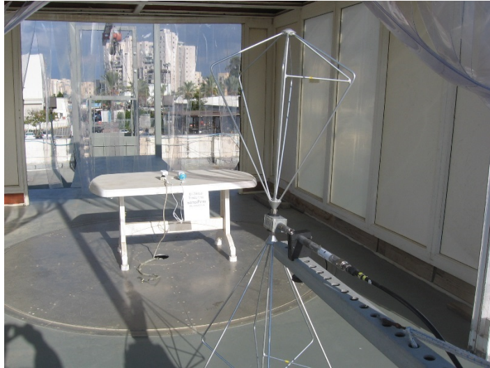
Radiated Emission Test 30-200 MHz
