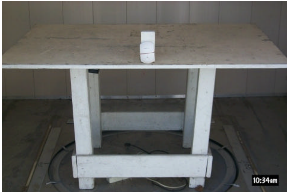
Figure 3.3 Radiated Test Setup, Z Axis
