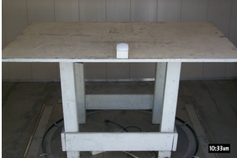
Figure 3.1 Radiated Test Setup, X Axis
