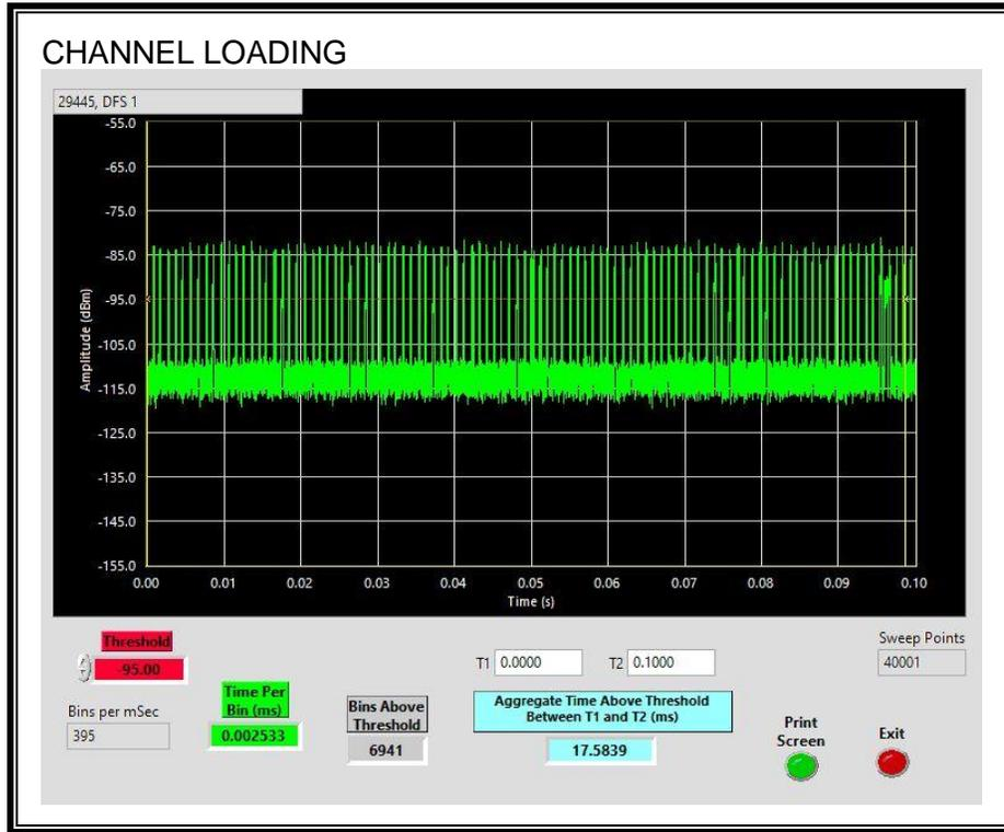
The level of traffic loading on the channel by the EUT is 17.58%
