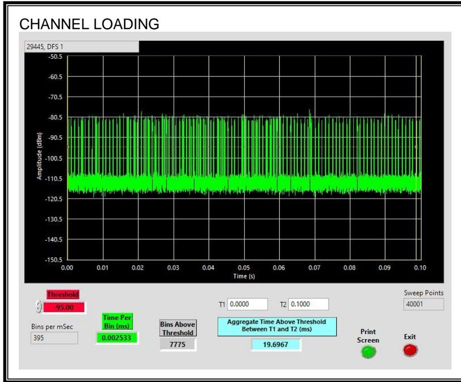
The level of traffic loading on the channel by the EUT is 19.69%
