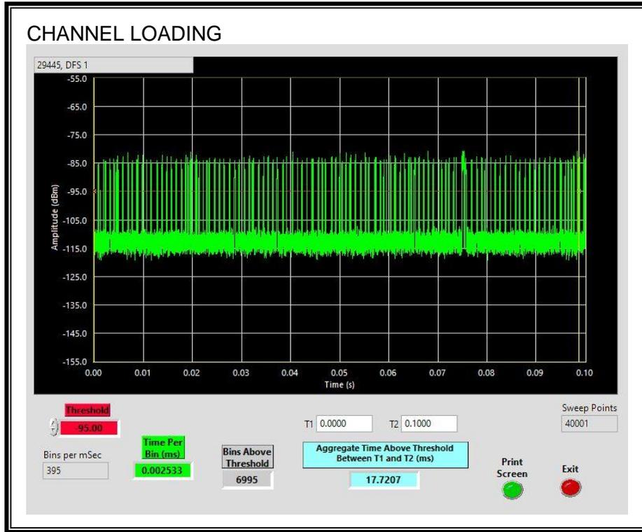
The level of traffic loading on the channel by the EUT is 17.72%
