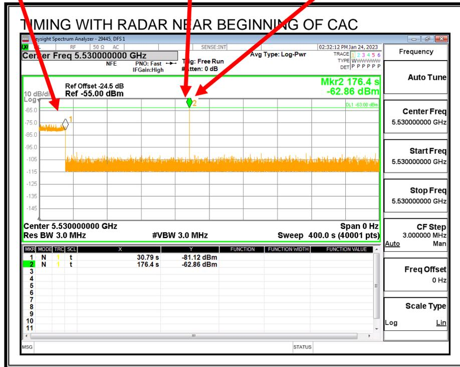
No EUT transmissions were observed after the radar signal.
