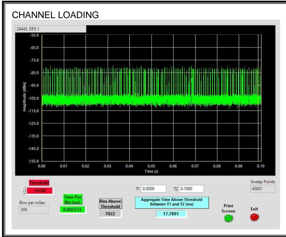
The level of traffic loading on the channel by the EUT is 17.78%
