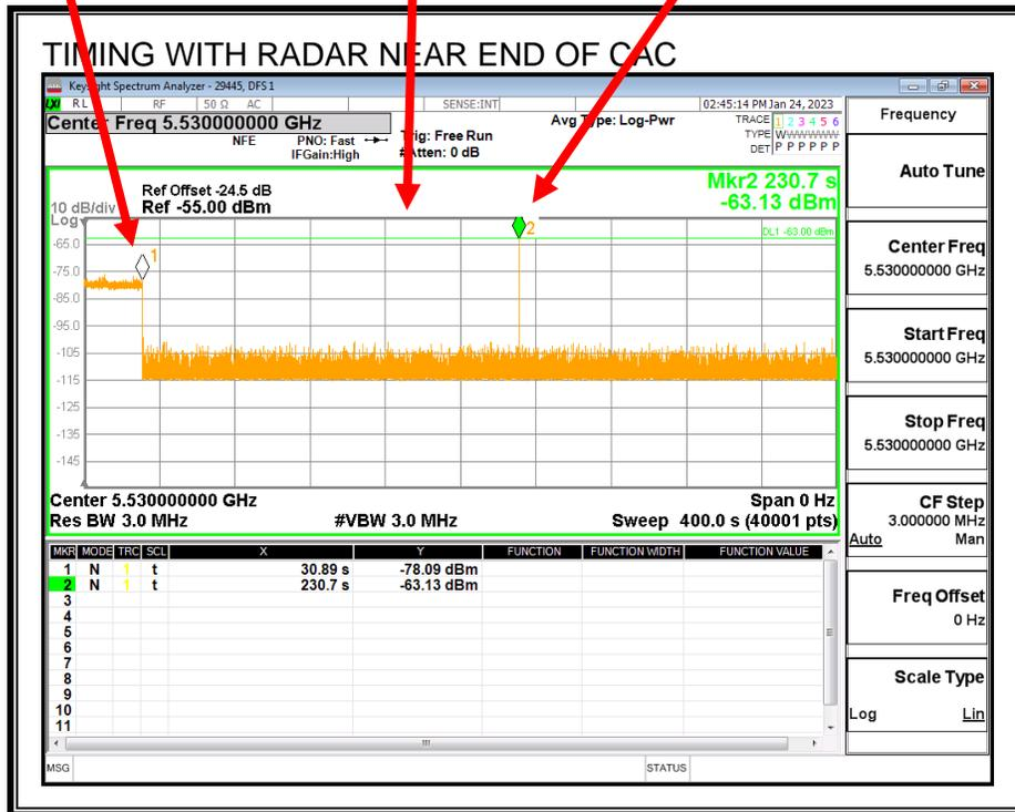
No EUT transmissions were observed after the radar signal.
