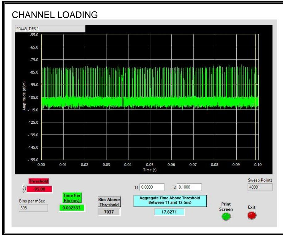
The level of traffic loading on the channel by the EUT is 17.82%
