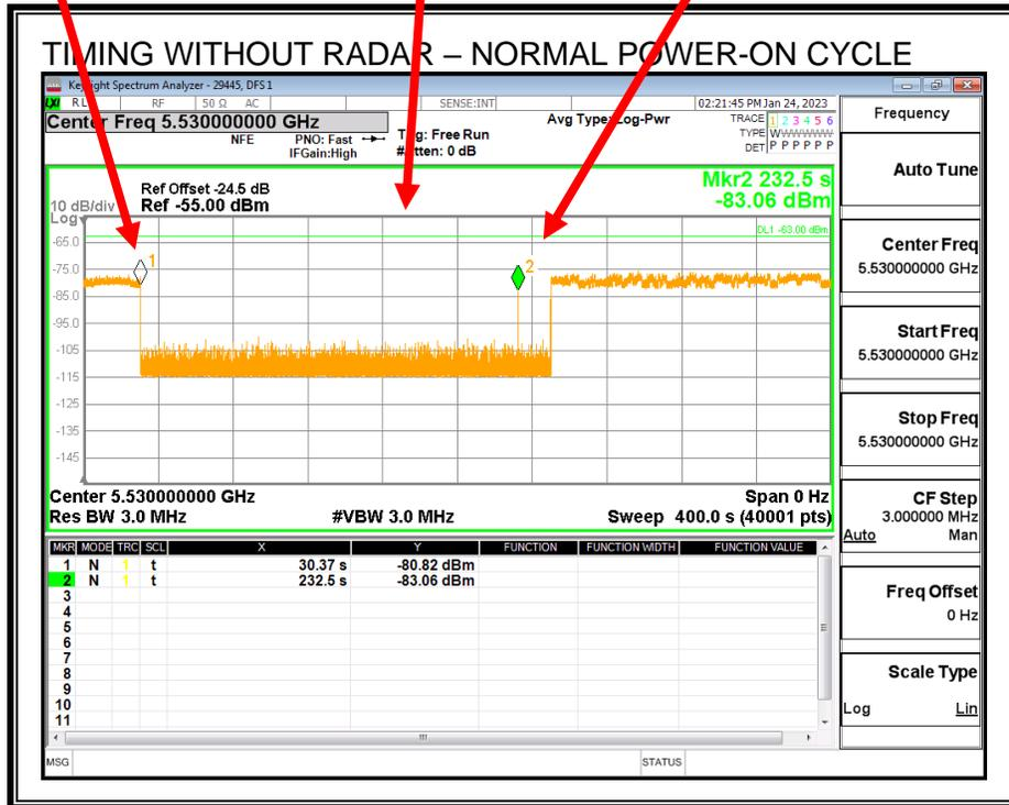
Transmissions begin on channel after completion of the initial power-up cycle and the CAC.
