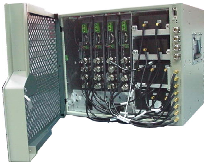
Figure 4-3. RC Open Cabinet with Internal Cabling
