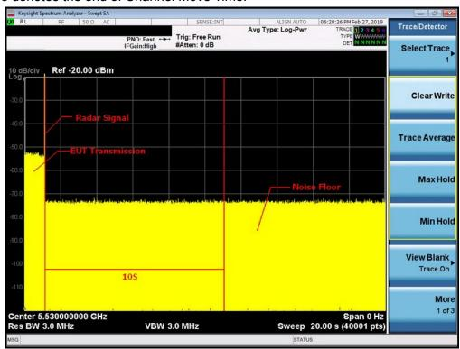
Note: An expanded plot for the device vacates the channel in the required 500ms
