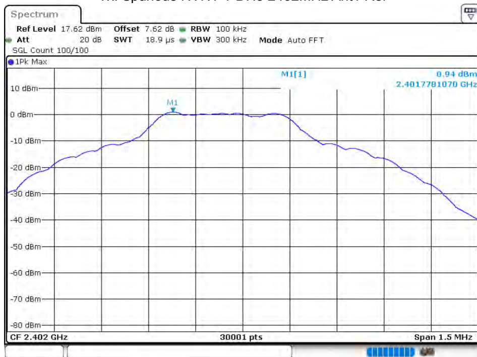
Tx. Spurious NVNT 1-DH5 2402MHz Ant1 Ref
