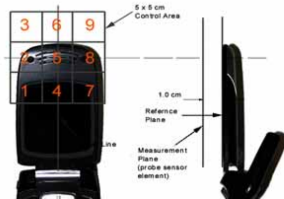
Figure 13 E/H-Field Emissions Test Setup Diagram
