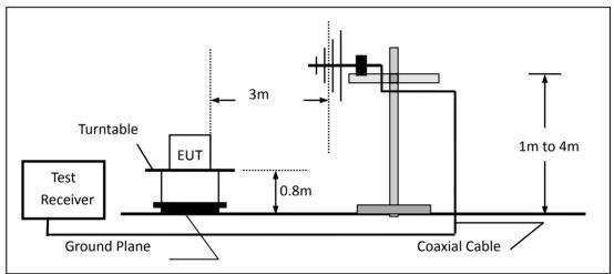
(c) For radiated emissions above 1000MHz
