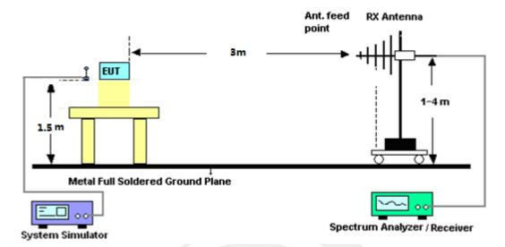
For radiated test from above 1GHz
