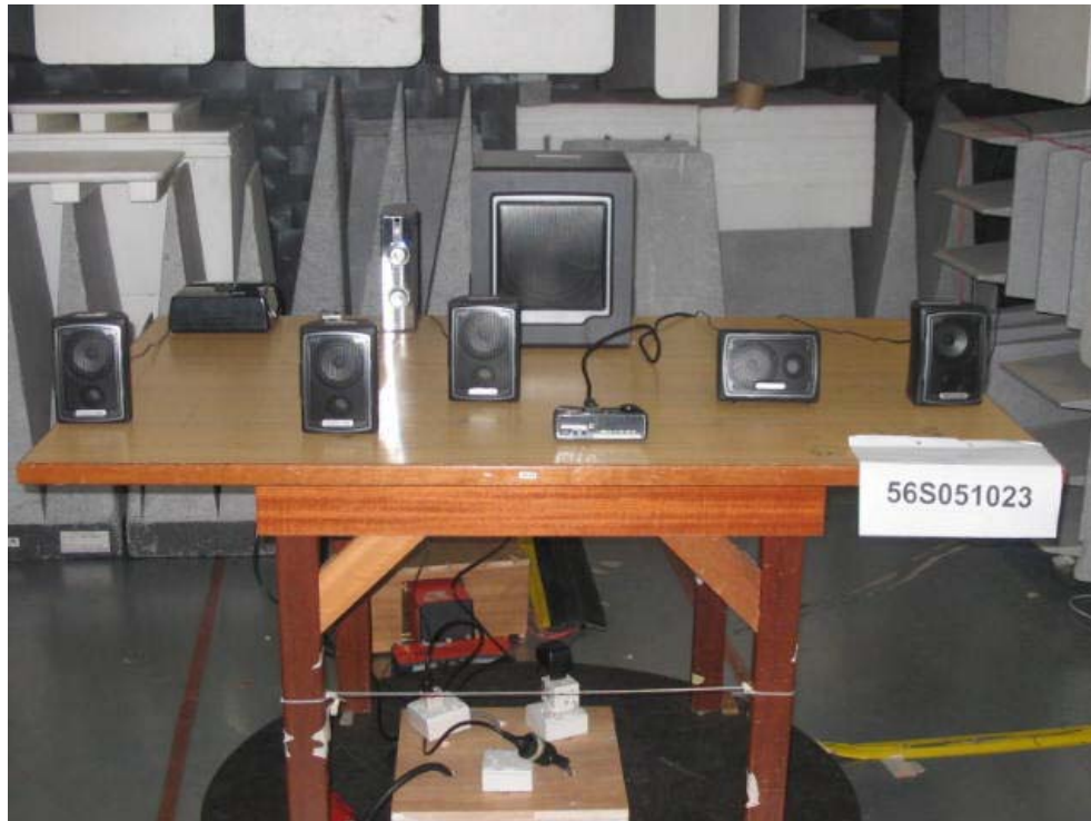
Radiated Emissions Test Setup (Front View)
