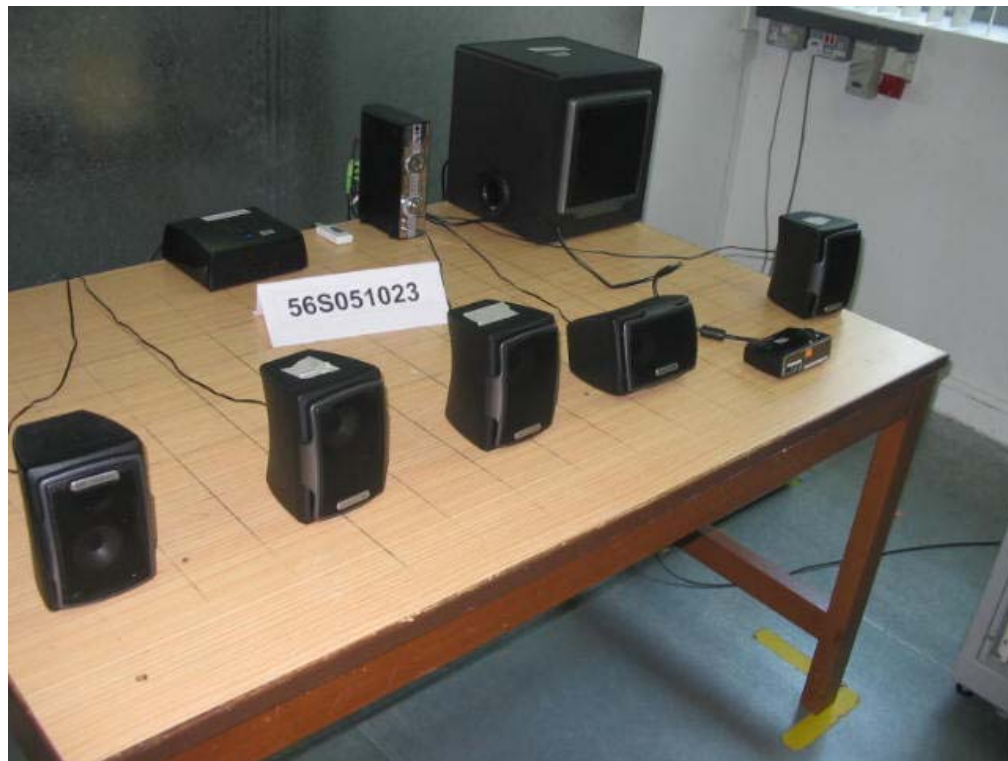
Conducted Emissions Test Setup (Front View)
