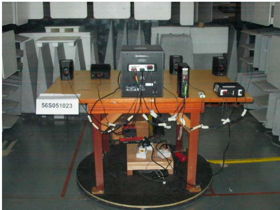
Radiated Emissions Test Setup (Rear View)
