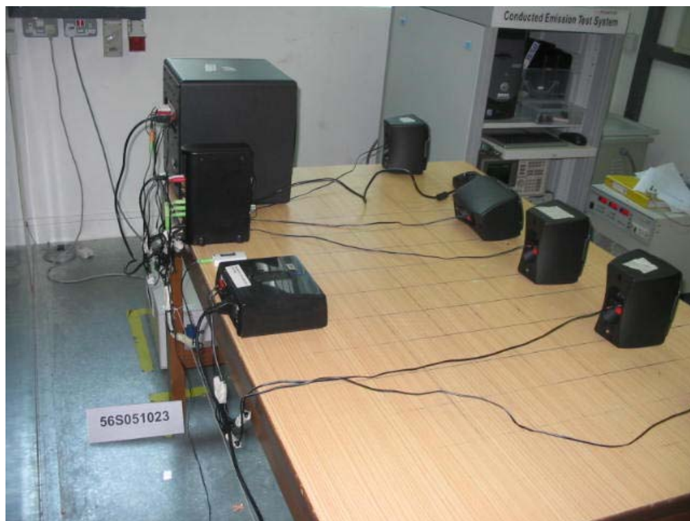
Conducted Emissions Test Setup (Rear View)
