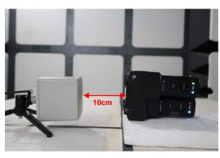
The Field Probe is placed 10cm distance to the front surface of EUT
