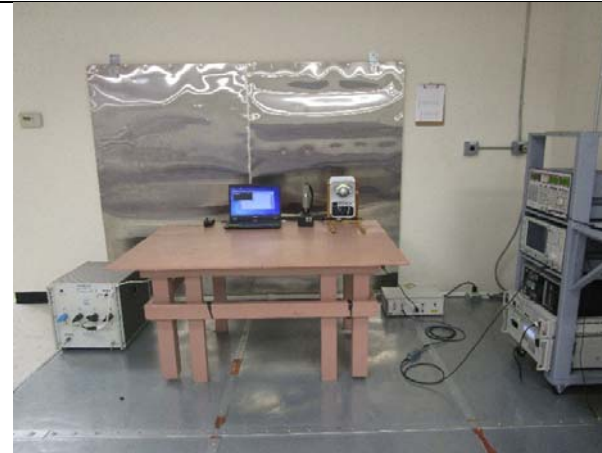
AC Line Conducted Emission – Front View
