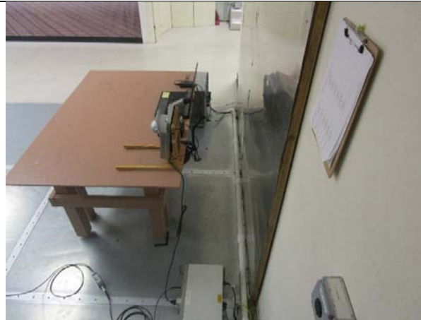
AC Line Conducted Emission – Rear View
