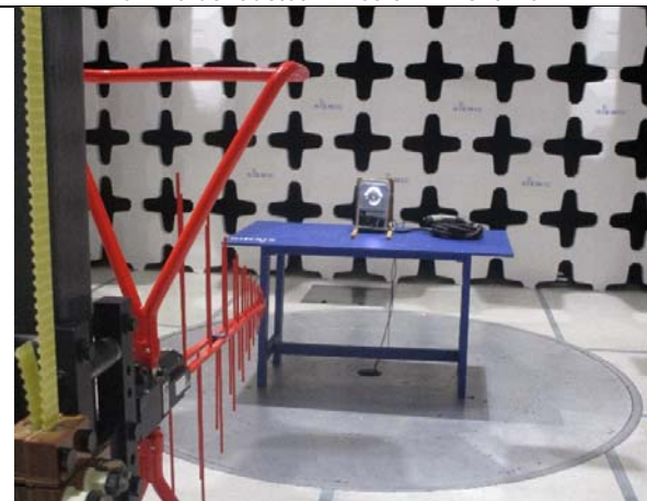
Radiated Emissions (<1GHz) – Front View
