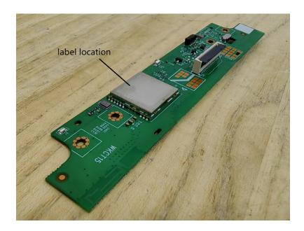
The label is attached to the surface of the shield with a permanent adhesive.
