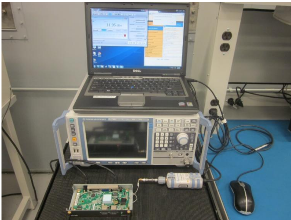
Figure B.2 - Conducted Measurement Test Setup 2 (Average Power Measurement)
