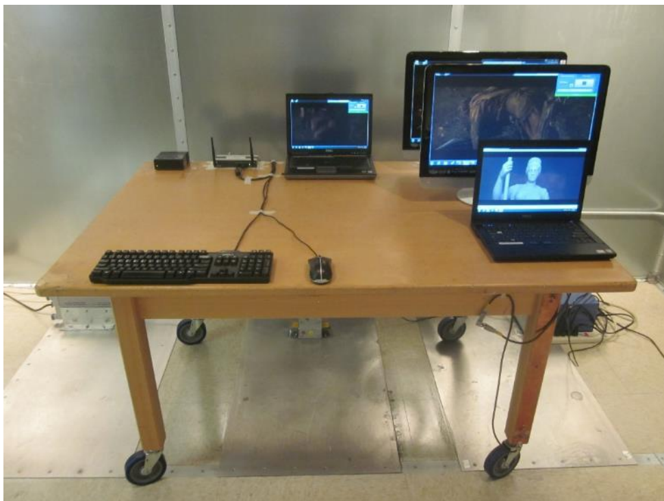
Figure B.6.4 - Conducted Emissions Test Setup - Front View; PoE PS
