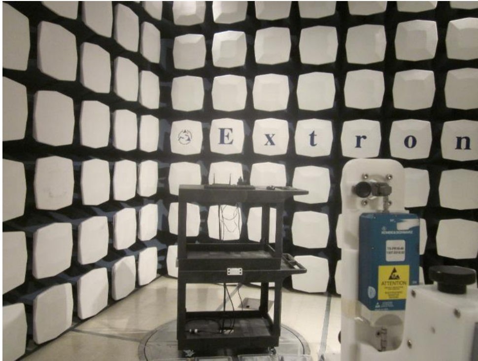
Figure B.4.1 - Radiated Emissions Test Setup - Front View; 18 GHz-40 GHz
