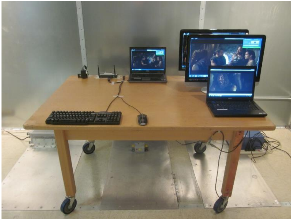
Figure B.6.1 - Conducted Emissions Test Setup - Front View; 5Vdc PS
