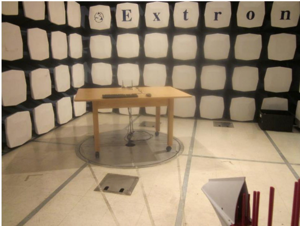
Figure B.2.3 - Radiated Emissions Test Setup - Front View; 30 MHz-1000 MHz; PoE PS
