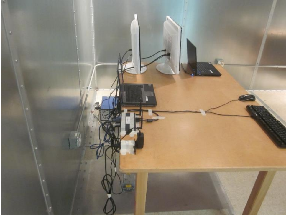
Figure B.6.3 - Conducted Emissions Test Setup - Side View 2; 5Vdc PS
