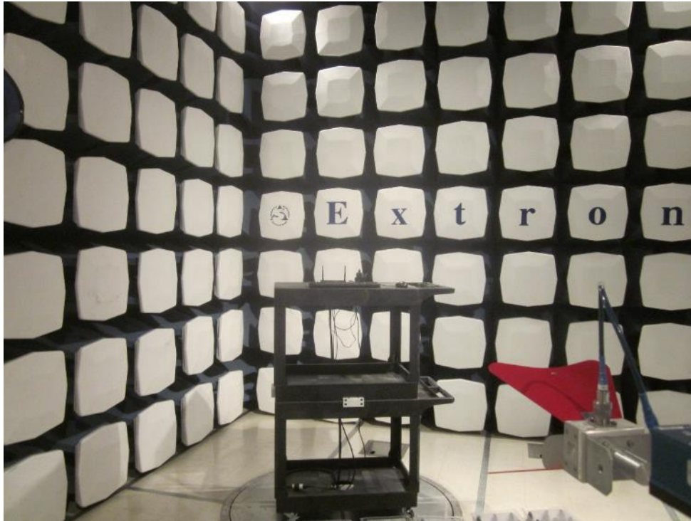
Figure B.3.1 - Radiated Emissions Test Setup - Front View; 1 GHz-18 GHz
