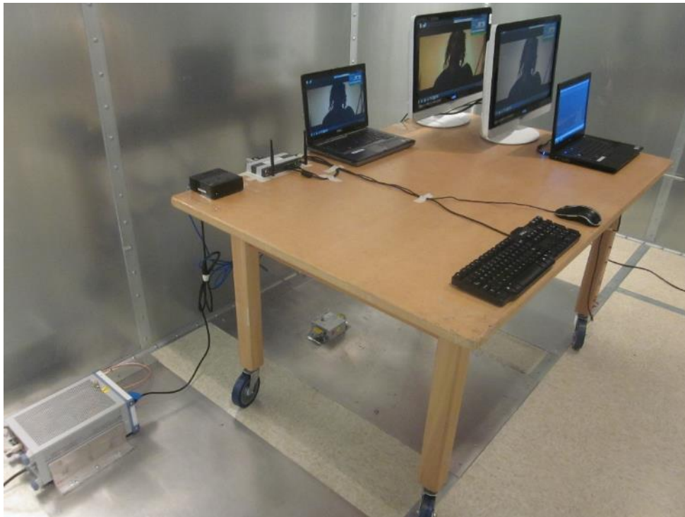
Figure B.6.5 - Conducted Emissions Test Setup - Side View 1; PoE PS
