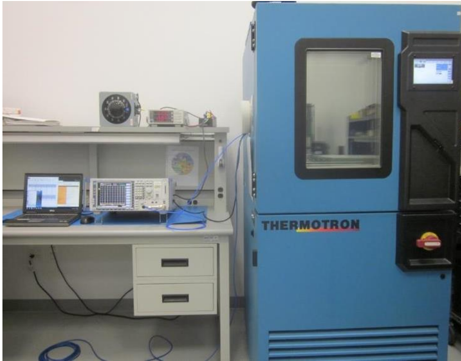
Figure 7.1 Frequency Stability Test Setup View 1
