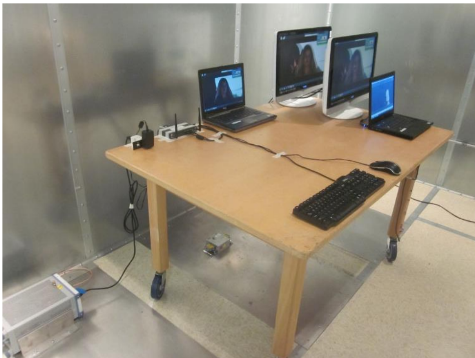
Figure B.6.2 - Conducted Emissions Test Setup - Side View 1; 5Vdc PS
