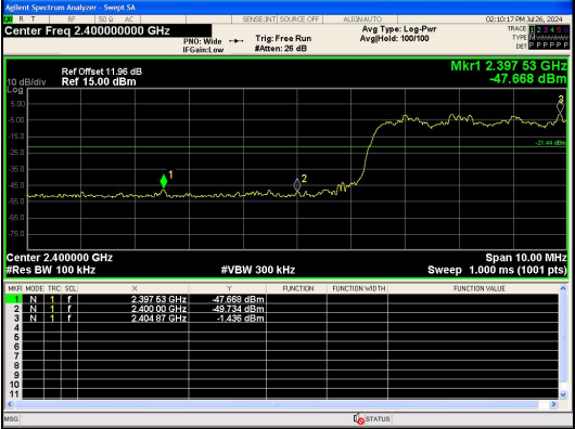
Out Of Band Emission(Left) \pi/4 DQPSK_2-DH5_Channel Hopping
