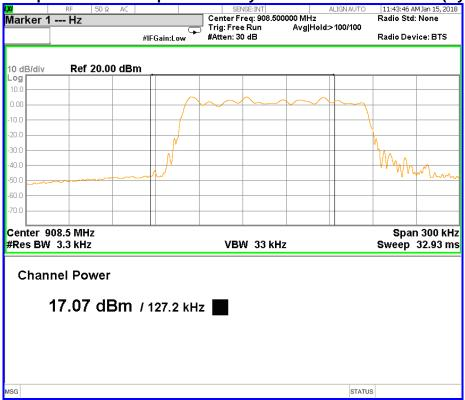
Screen Captures from the spectrum analyzer: 125 KHz High Channel (Hybrid Mode)
