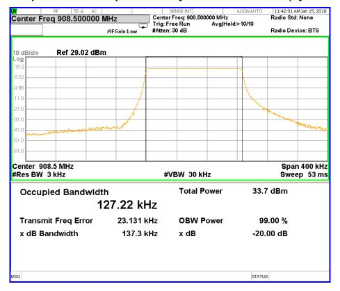
Screen captures from the spectrum analyzer 125 KHz Channel (Hybrid Mode)
