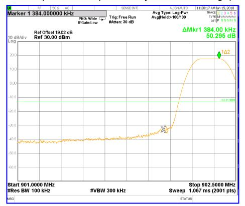
Screen Capture from the spectrum analyzer: Upper Band Edge (125 KHz)
