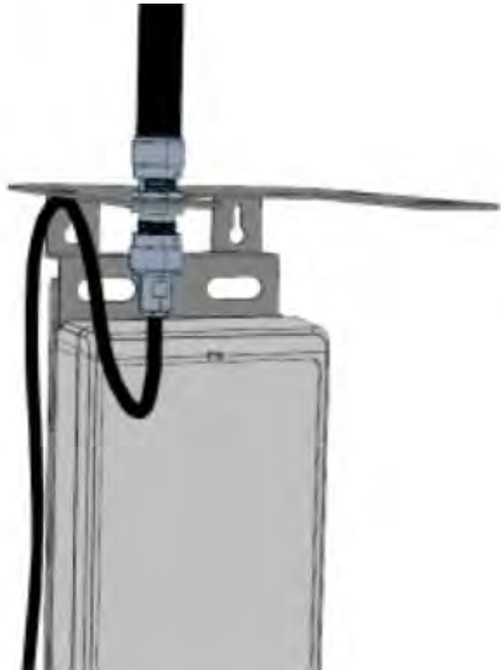
Figure 20: Gateway's antenna mounting.
