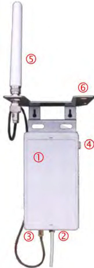
Figure 13: LS-G6 Gateway, with all the parts indicated.
