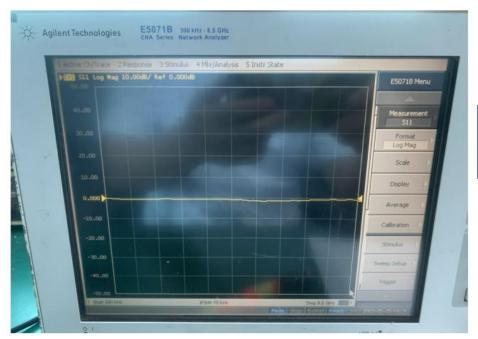
The Agilent E5071B network analyzer is mainly used for passive 2D/3D antenna testing
