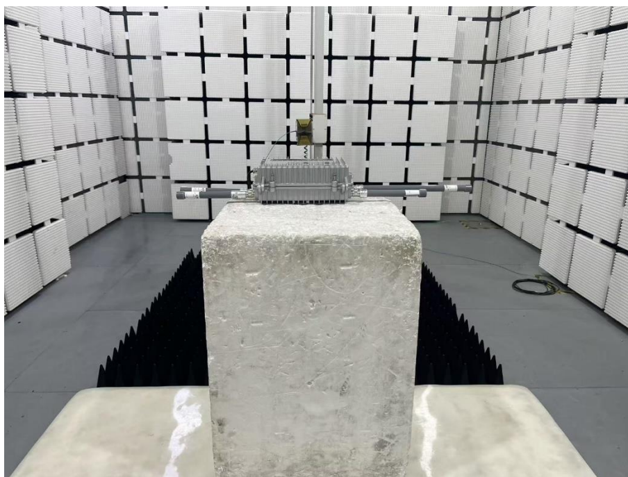
Set-up for Radiated Spurious Emission, Above 1GHz
