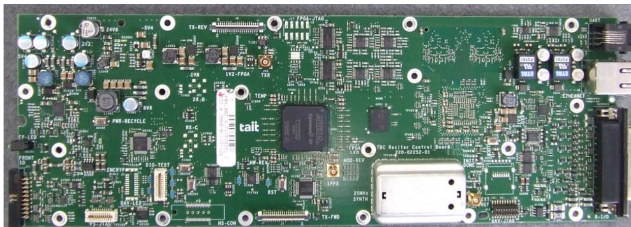
Photograph 10: Reciter Control Board (RCB) – Top
