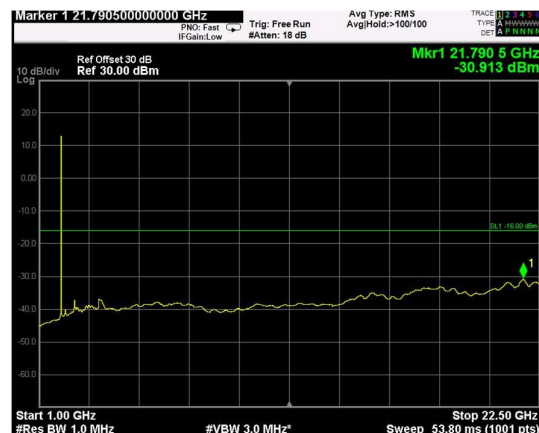
Channel: TOP, Modulation: 64QAM, BW=10MHz, Range: Upper
