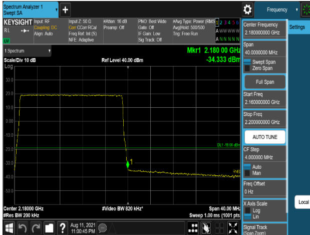
Plot 7-997. Band Edge Emission (2180MHz to 2181MHz) Plot (B66_5M+5M+5M+20M_4C_QPSK - High Channel, Port 3)
