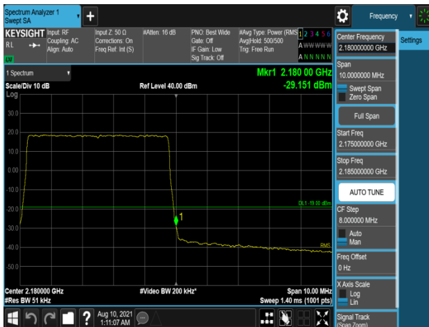
Plot 7-969. Band Edge Emission (2180MHz to 2181MHz) Plot (B66_5M+5M_2C_QPSK - High Channel, Port 2)
