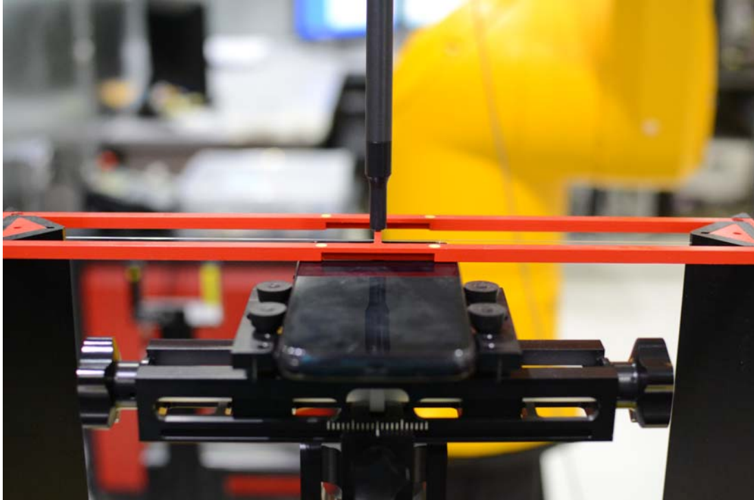
Figure 18-1 Ear Reference Point HAC Phantom Alignment
