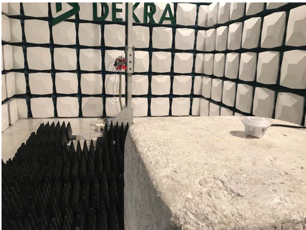
Description: Radiated Emission Test Setup for 1~18GHz
