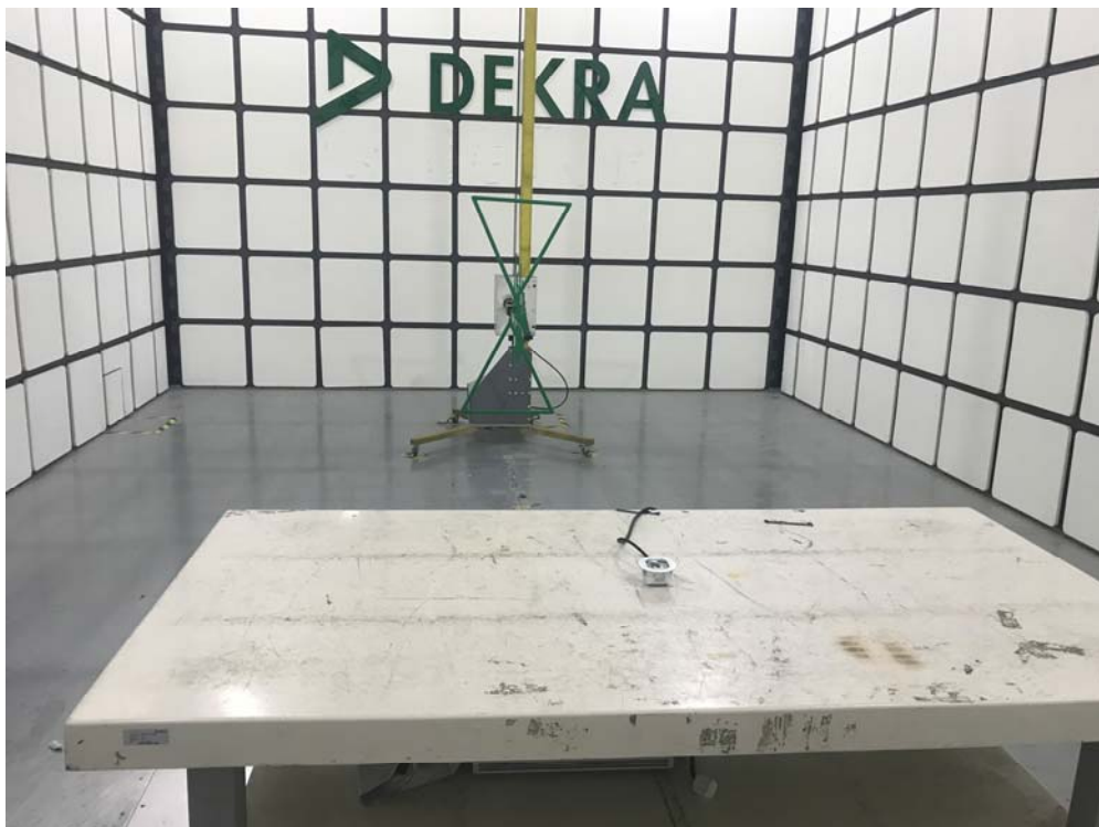
Description: Radiated Emission Test Setup for 1~18GHz
