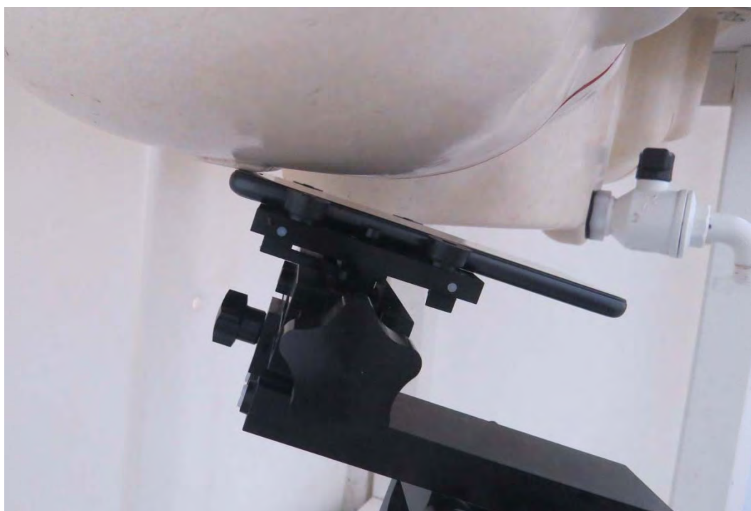
Picture 19: Right Hand Tilt 15 Degree Position
