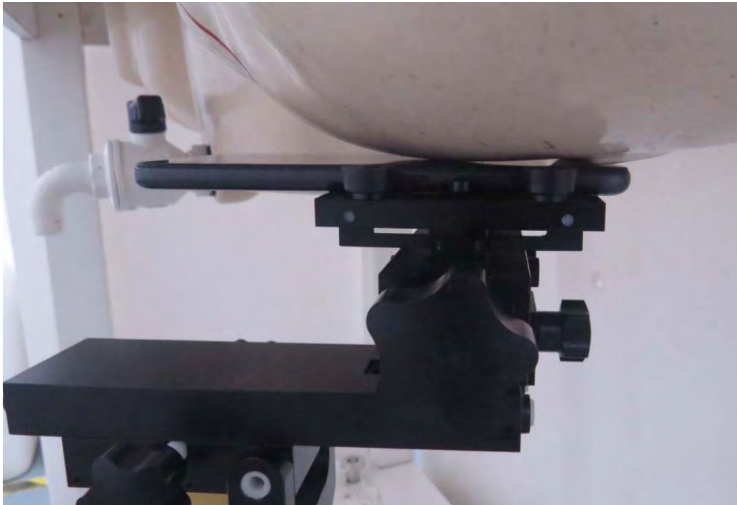
Picture 16: Left Hand Touch Cheek Position
