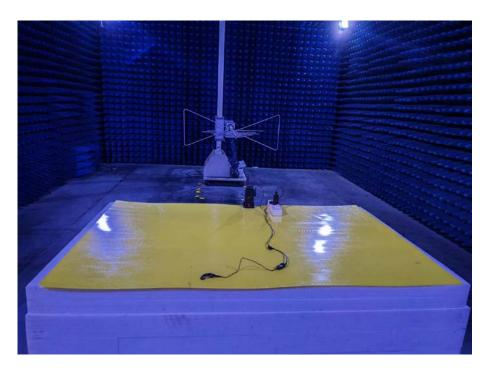
Radiated Emissions – Test mode 2 (Below 1 GHz)
