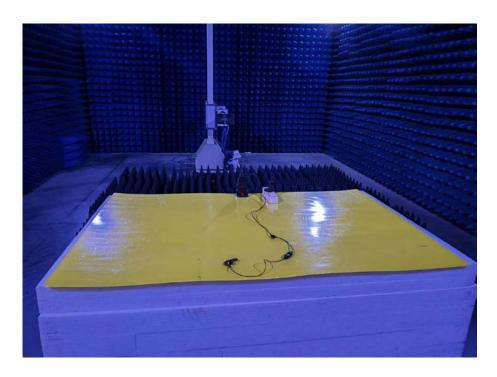
Radiated Emissions – Test mode 2 (Above 1 GHz)
