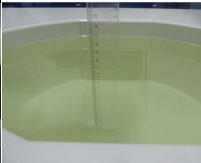
Photo 8: 2450MHz Liquid Depth \geq 15.0\text{cm}
