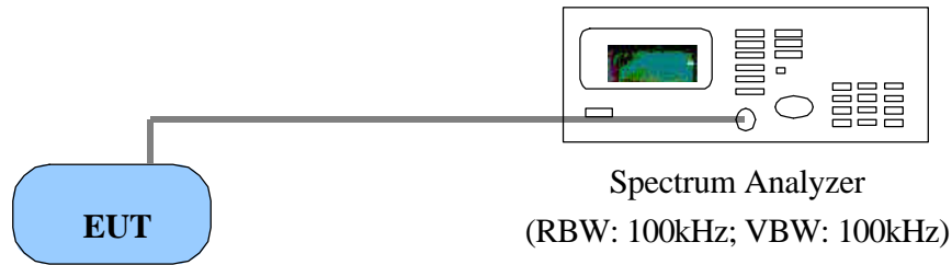
Test Configuration of Bandwidth for Direct Sequence System
