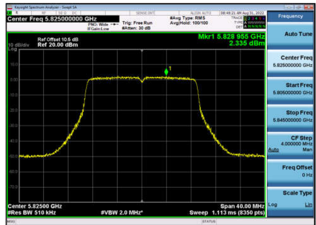
U-NII-3 Power spectral density-802.11 n(40MHz),5755MHz,Ant1
