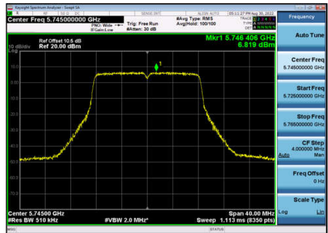
U-NII-3 Power spectral density-802.11 a(20MHz),5785MHz,Ant1
