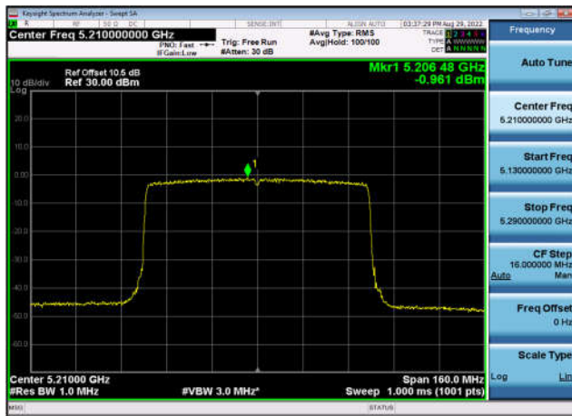
U-NII-3 Power spectral density-802.11 n(20MHz),5745MHz,Ant0
