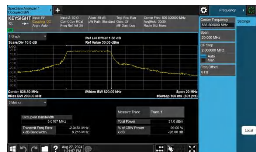
Band26(824-849)-10MHz-16QAM-26915-27RB#0-PASS
