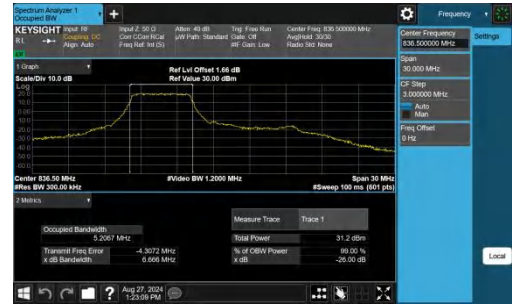
Band26(824-849)-15MHz-16QAM-26915-27RB#0-PASS
