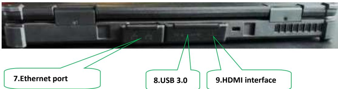
**7.Ethernet port:** RJ45 port, user can link internet to using in this.
