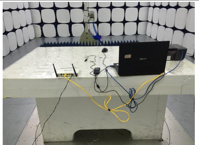
Radiated Emissions Test Setup Above 1GHz
