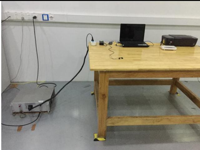
Conducted Emissions Test Setup – Front View
