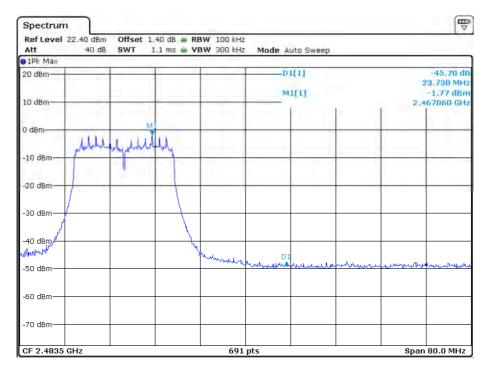
802.11n-HT40 Channel 03 (2422MHz) Reference Level: -6.68dBm
