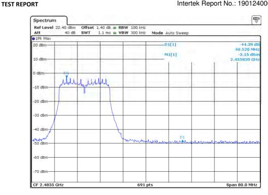
802.11n-HT40 Channel 03 (2422MHz) Reference Level: -7.75dBm
