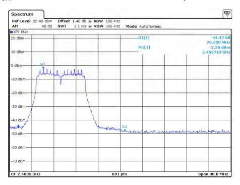
802.11n-HT40 Channel 03 (2422MHz) Reference Level: -6.50dBm
