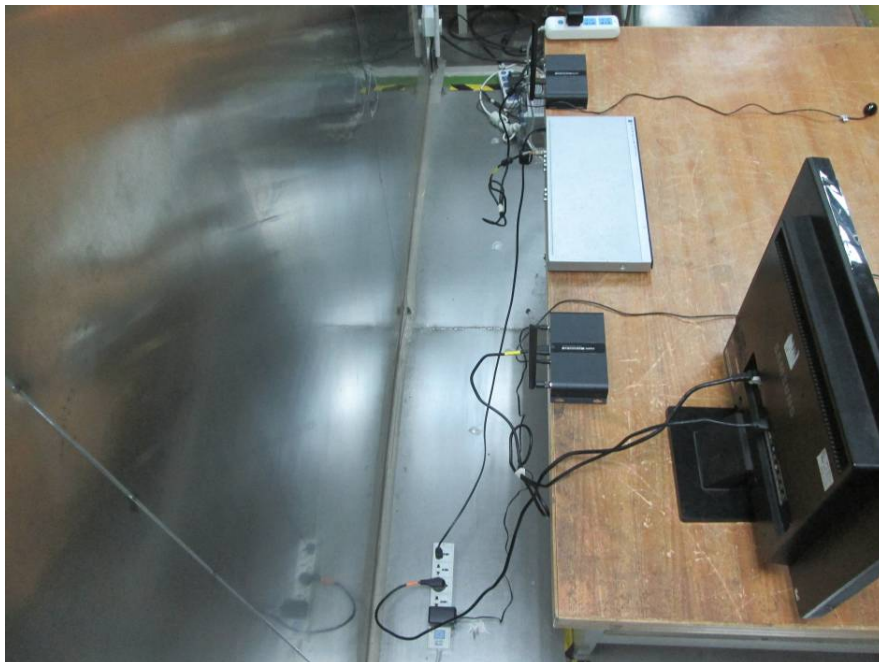
Conducted Emissions - Side View
