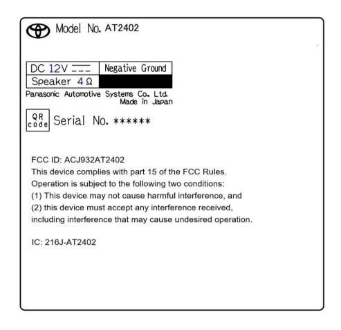
Label display: Printed on paper with ink using a printer and attached to the internal unit Durability of marking: Will withstand expected lifespan without peeling or fading FCC ID character size: 1.5mm
