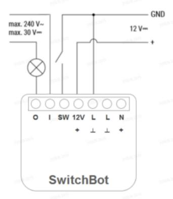
Complete the previous two steps. Instead of connecting the 12V+ to the + terminal, connect it to the 12V terminal.
